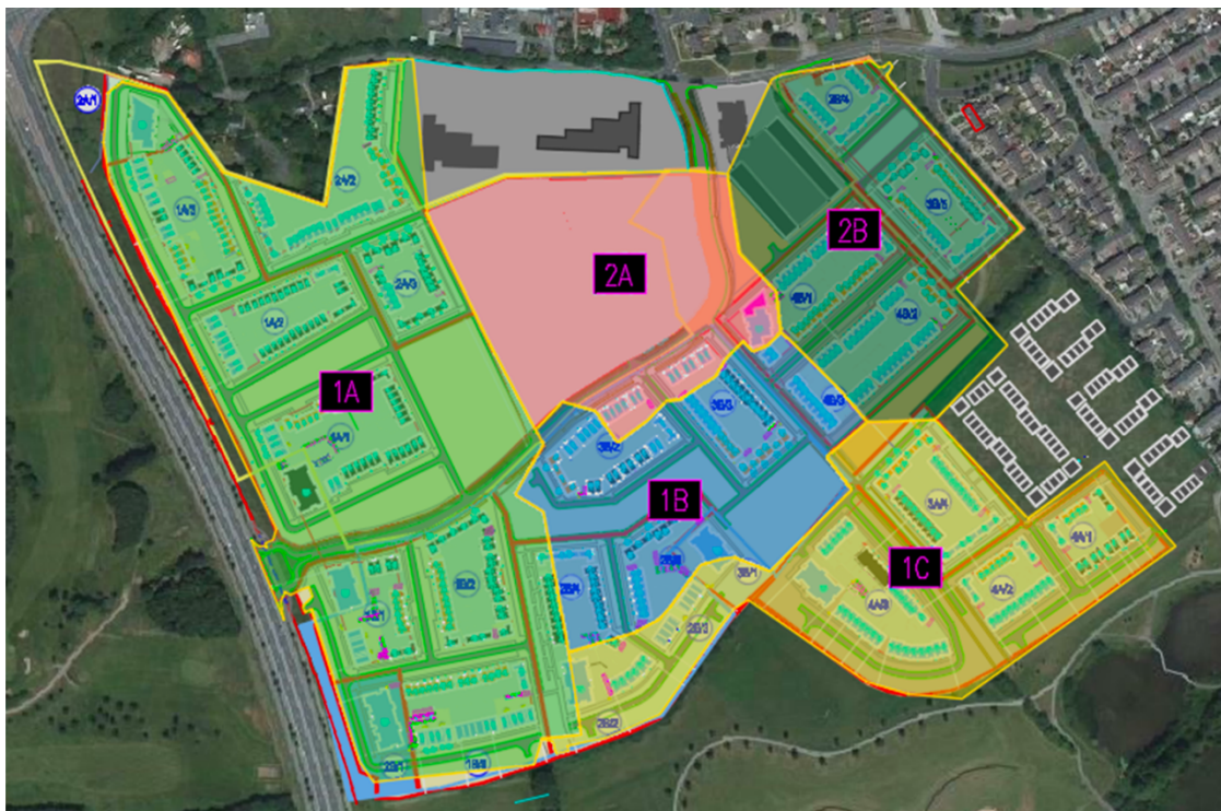
Figure 4: Extract from the Infrastructure Design Report, prepared by DBFL Consulting Engineers showing the surface water catchment areas across the site.
